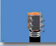
The screws will be mounted and the cable will be lowed
