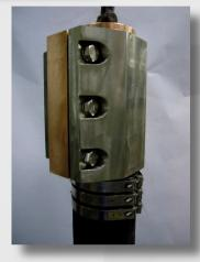
Once only, adapters will be installed at the contact surfaces of the electrode arm and the delta closure.
