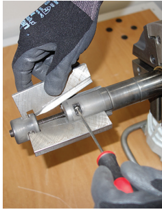
Fast adjustment of the pipe dimension
